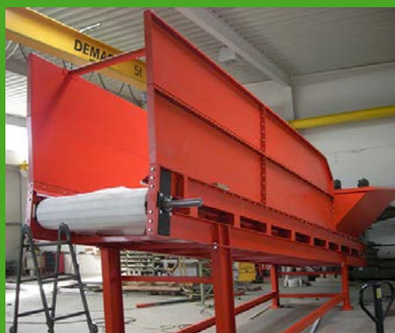
Conveyor belt with hopper
